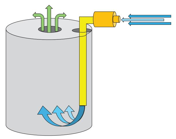
Negative-pressure ventilation pulled air from the space pulling in fresh air. When negative-pressure ventilation is used, position the exhaust so that hazardous air does not create a hazard to others.
